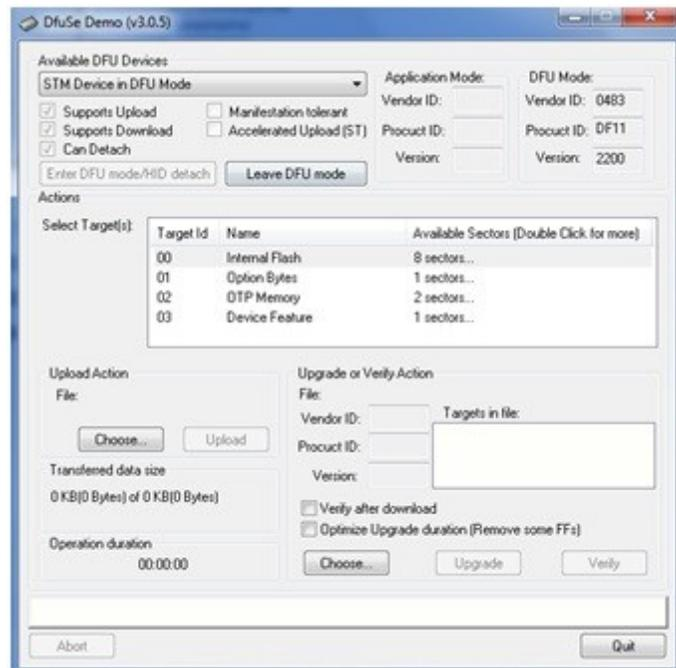
Press the button “Choose...” and select the previously prepared file with the extension .dfu. The window is converted to the form:
