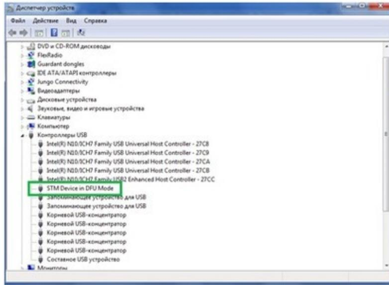
If this device is marked as undefined (with a yellow triangle), then you need to automatically search for drivers on your computer in the DfuSe Demo program folder. Next, you need to run the DfuSe Demo program. The following window will open:
