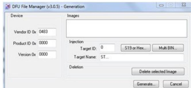
Click on the “S19 or Hex” button, find and select the firmware file Reciever\_msi001hex. Press the button “Generate ...”. The program will suggest a location to save the file with the .dfu extension. We indicate the desired file name and indicate the path for saving. A message like this will appear:
