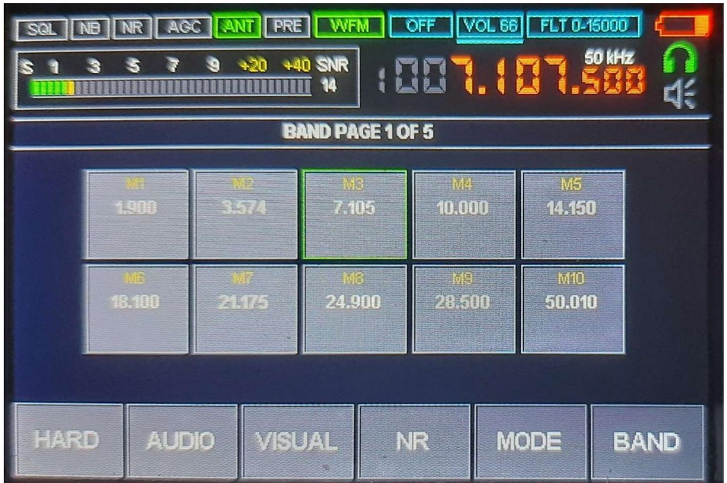
The BAND menu is used for selecting (recalling) or saving to a memory location, the current values, (including Frequency, MODE, etc.). Move around the pages by means of the encoder ENC\_FREQ. Exit is performed by pressing the BAND button or by pressing the ENC\_VOL encoder.
