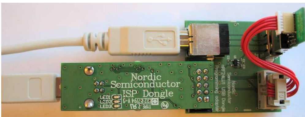
Figure 6 - nRF24LU1 USB Dongle Programming Adapter assembly
