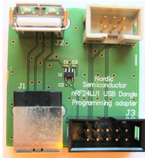
Figure 5 - nRF24LU1 USB Dongle programming adapter
