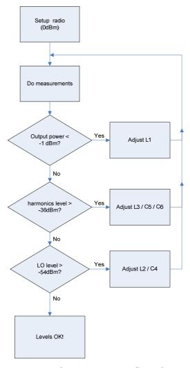
Figure 2- Measurement flow chart
