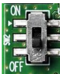
Figure 11: The actual Power supply switch (SW2)
