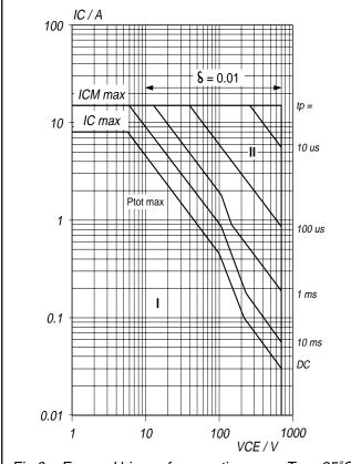
Fig.9. Forward bias safe operating area.  $T_{hs} = 25^{\circ}C$  Region of permissible DC operation.
