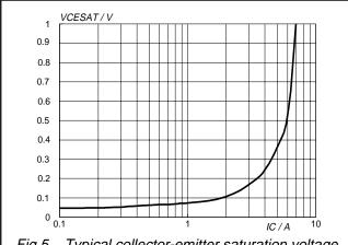
Fig.5. Typical collector-emitter saturation voltage.  $V_{CE}$ sat =  $f(I_C)$ ; parameter  $I_C/I_B$
