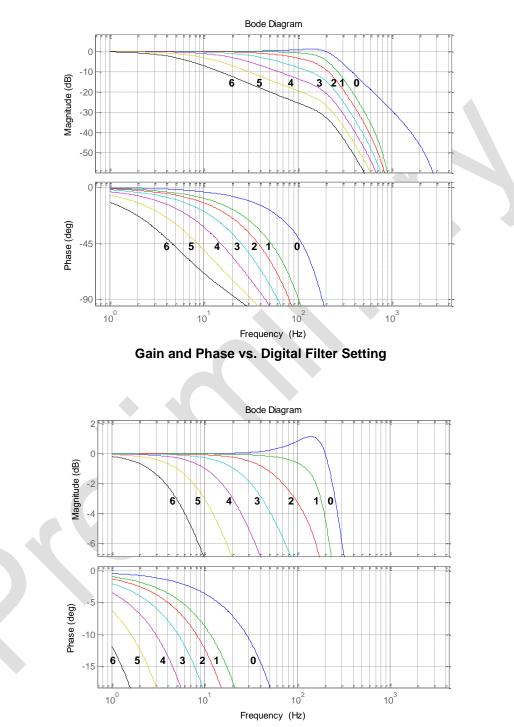
Gain and Phase vs. Digital Filter Setting, Showing Passband Details
