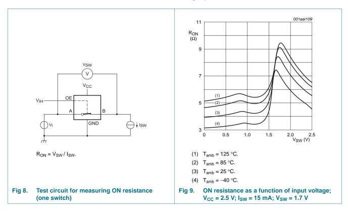
Measured by the voltage drop between the A and B terminals at the indicated current through the switch. ON-state resistance is determined by the lower of the voltages of the two (A or B) terminals.
