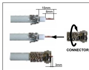
3.1 On a coax cable approximately 1,5 m long, set up two F connectors and connect the LNB to the rotor's LNB plug. Fit an F-connector on each end of the cable going to the receiver and connect the rotor's REC plug to the plug of your receiver.
