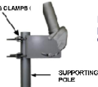
Fix the rotor to the supporting pole without tightening definitively the brackets.
