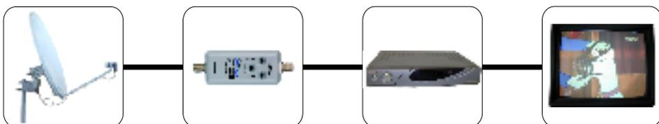
**MP01 Mini-pos configuration for DiSEqC 1.2 receivers without reset (Go to 0).
