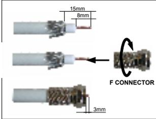
On a coaxial cable approximately 1,5 m long, set up 2 F-connectors and connect the LNB to the rotor's LNB plug.
