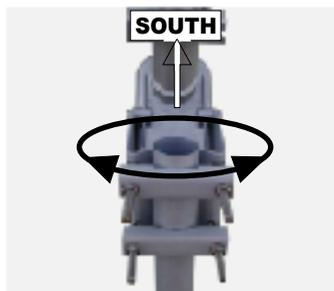
2.2 Align the dish to rotor's pole indicator.
