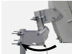
**7.5 Case nr 4** - If the picture quality improves while bending the dish downwards/both eastwards and westwards, you should loosen the rotor's fixing screws and increase slightly the elevation on the bracket. Find the best picture and store the new position. Now you can operate the recalculation (if your receiver gets the function). If not, you have to go back to each memorized position, check the best picture and store all positions one by one.
