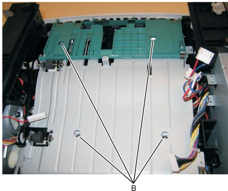
7. Lift the duplex slightly, push to the left, and tilt to clear the right side of the printer.
