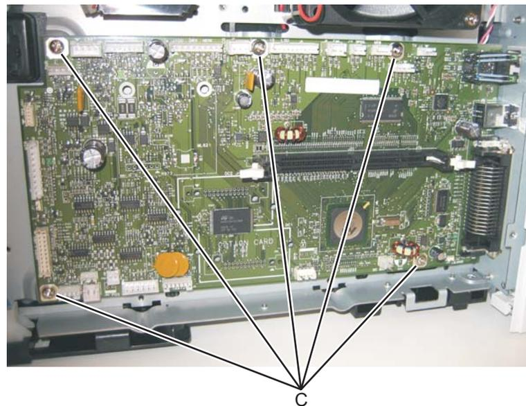
5. Lift the controller board, and remove.
