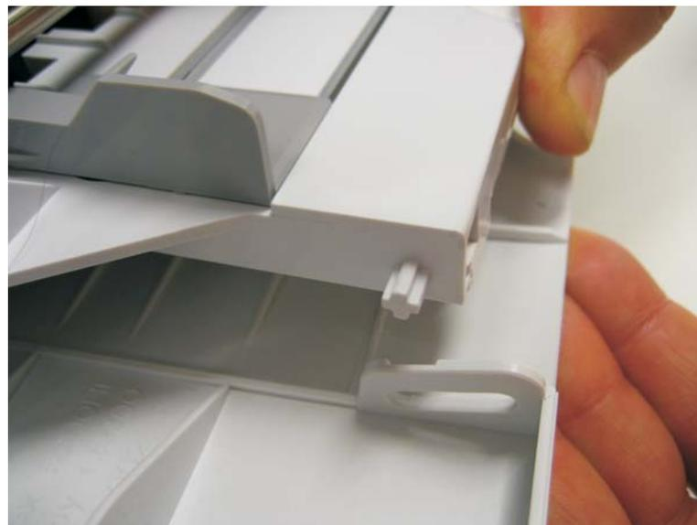
6. Disconnect the fuser link (A) from the front access door.
