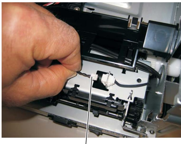
7. Disconnect the exit sensor cable (E) from the controller board.
