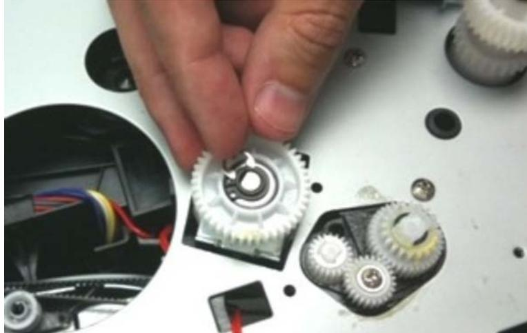
4. Pull up the clutch from the cavity, exposing the white tape.
