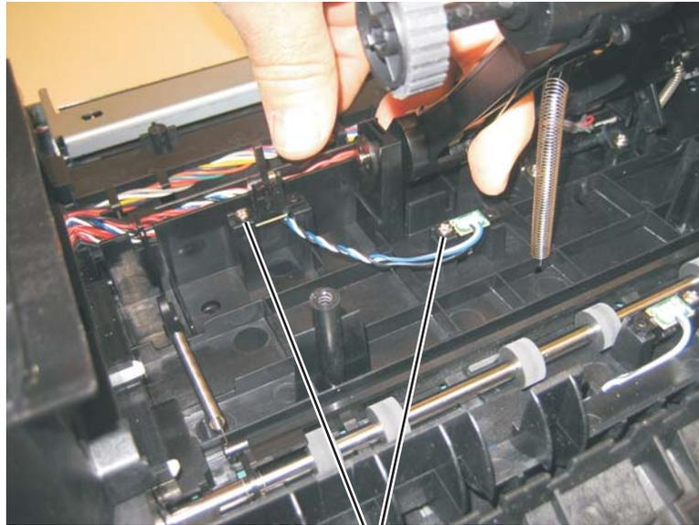
4. Disconnect the sensor cable (B) from the controller board.
