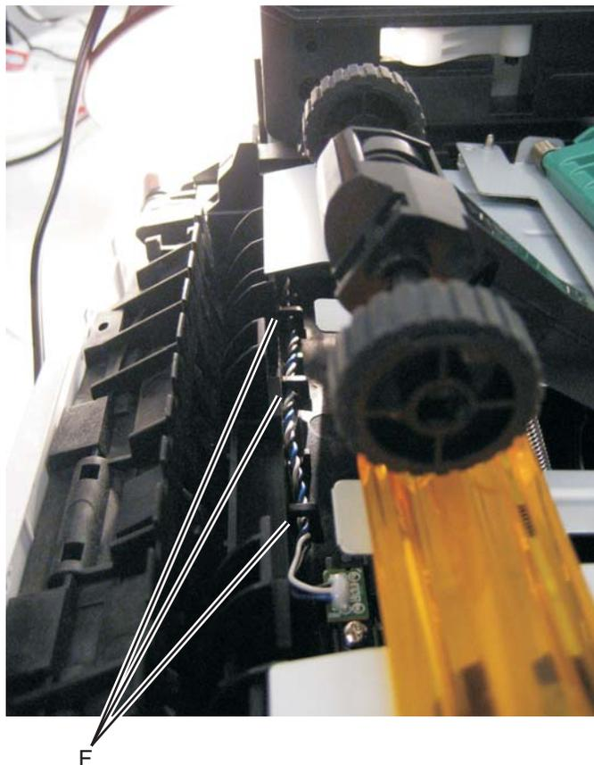
**Note:** If the cable is not properly installed in its retainers, then the loose cable will obstruct the paper path.
