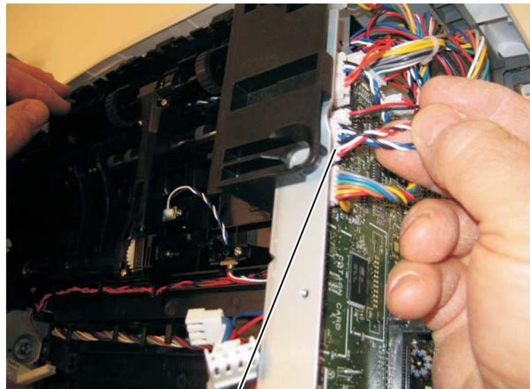
5. Remove the paper input and duplex sensor assembly.
