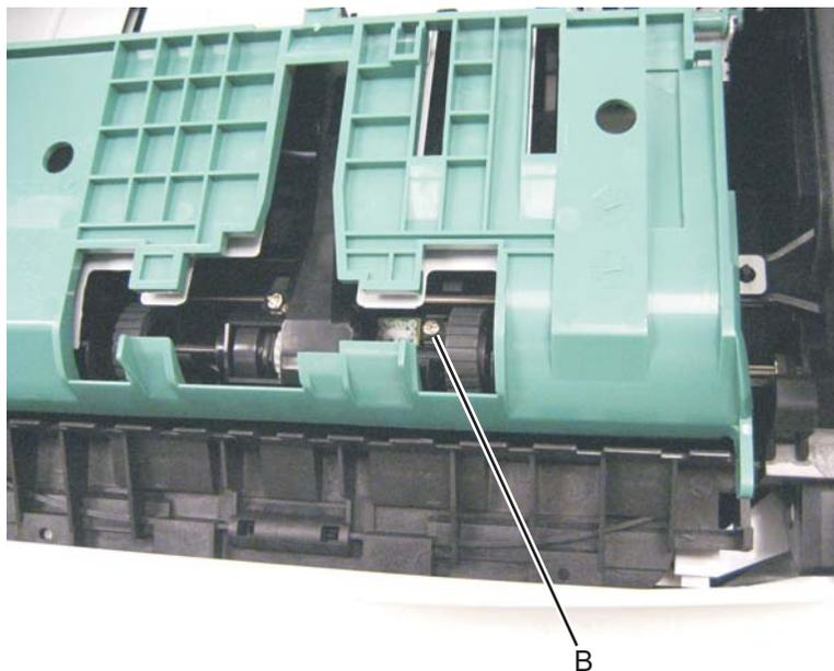
5. Free the cable from its retainers, and pull it through the opening toward the sensor mount.
