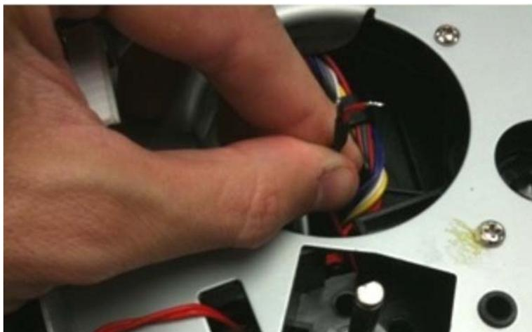
8. Remove any shrink tubing that is holding the wires together.
