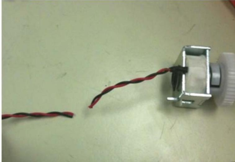
3. Install the new media clutch on the ACM drive shaft.
