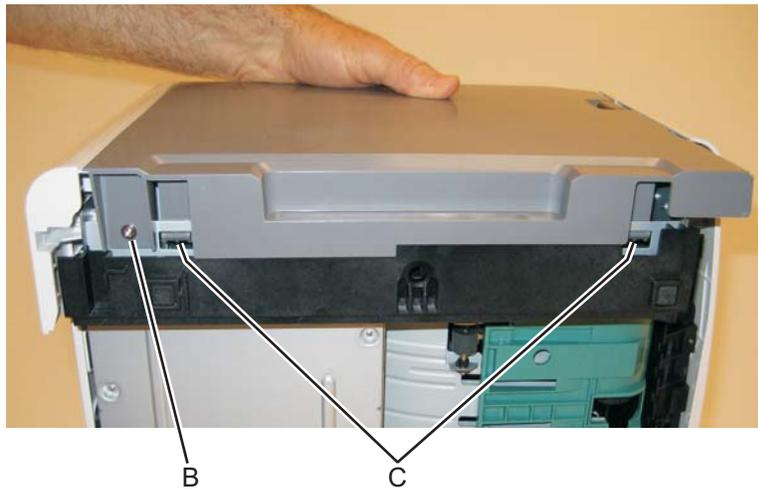
4. Rotate the cover out, and lift to remove the left side cover.
