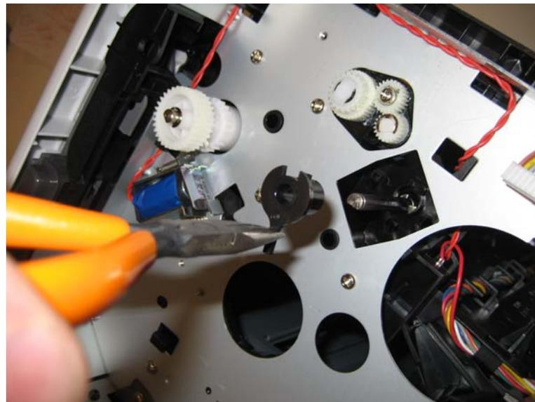
8. Use a screwdriver to pop the inner shaft lock (B) loose.
