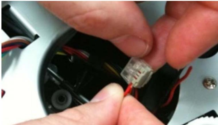
5. Insert the red wire from the clutch into the wire splice connector.
