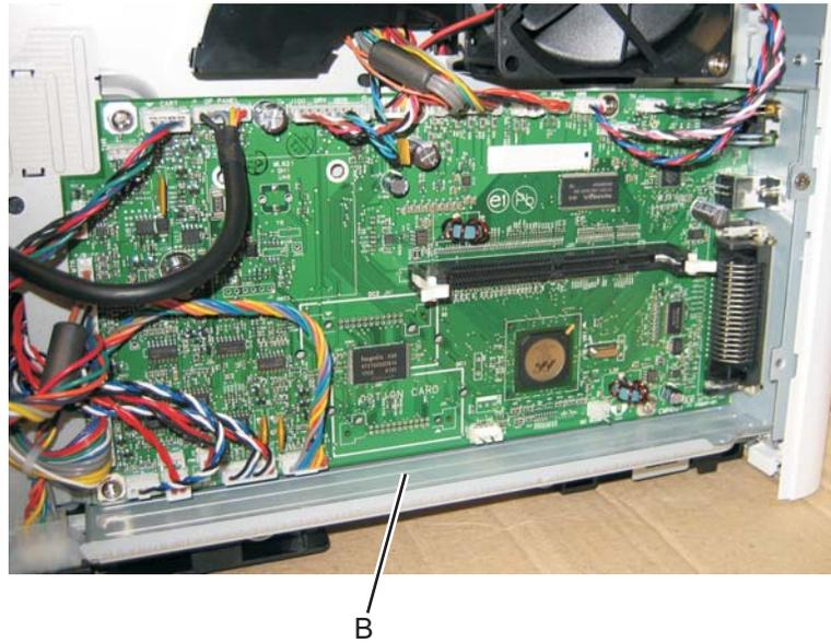
4. Remove the five screws (C) from the controller board.
