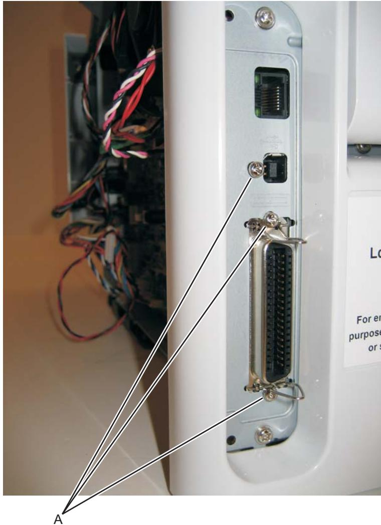
3. Disconnect all of the cables from the controller board.
