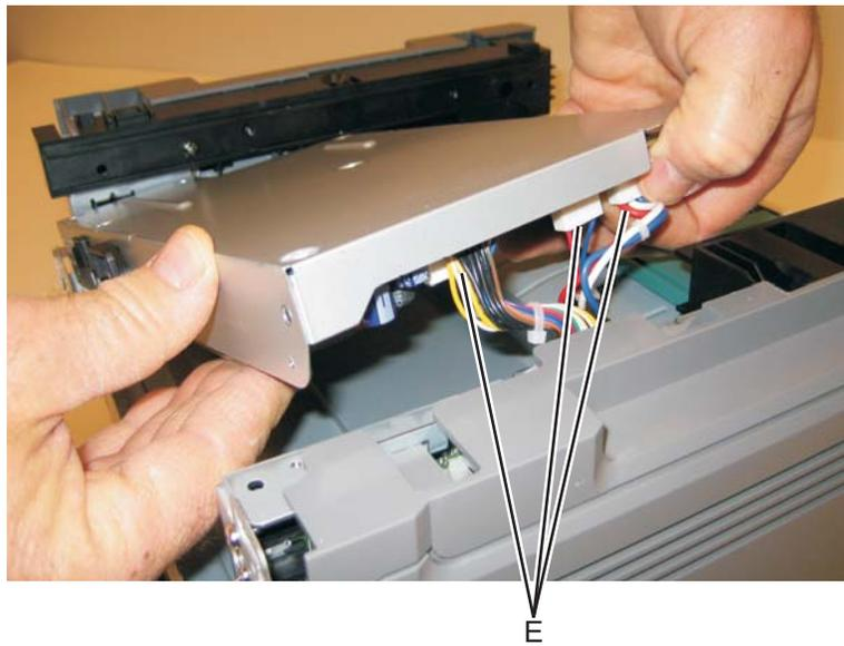
**Note:** Squeeze the clip to remove the cables from their connectors (F).
