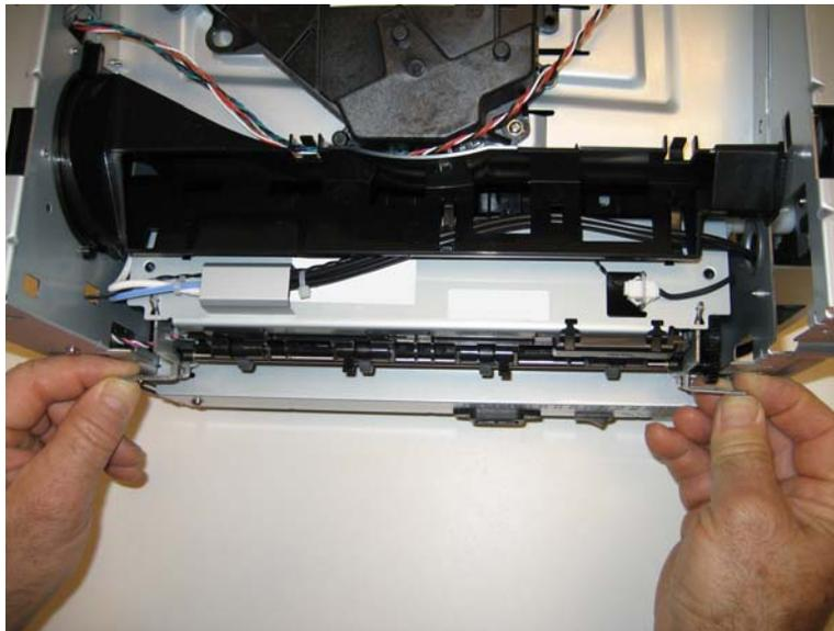
4. Push in on the cable connector cover (B), and remove.
