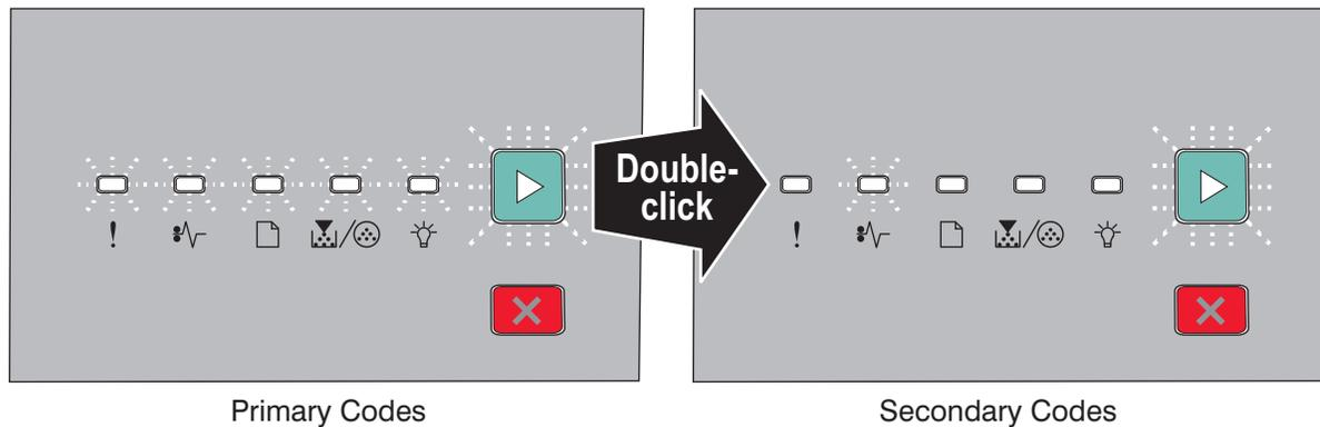
All service errors are indicated by all lights flashing as the primary notification or code. The secondary code indicates an area or function which has the error. Additional tertiary codes used for service (see **“Service tertiary error codes” on page 2-30**) indicate specific errors. See **“Service codes” on page 2-28**.
