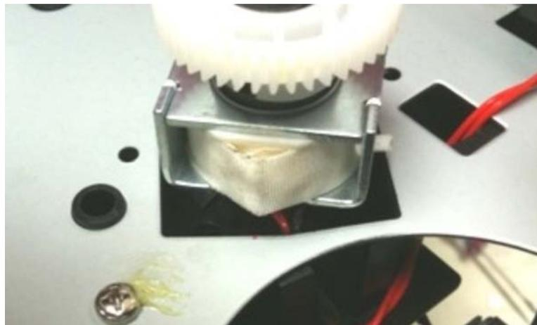
6. Clean any adhesive residue from the wires.
