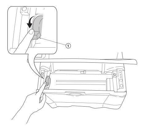
Figure 2-2-1 Confirming the lock lever #1
