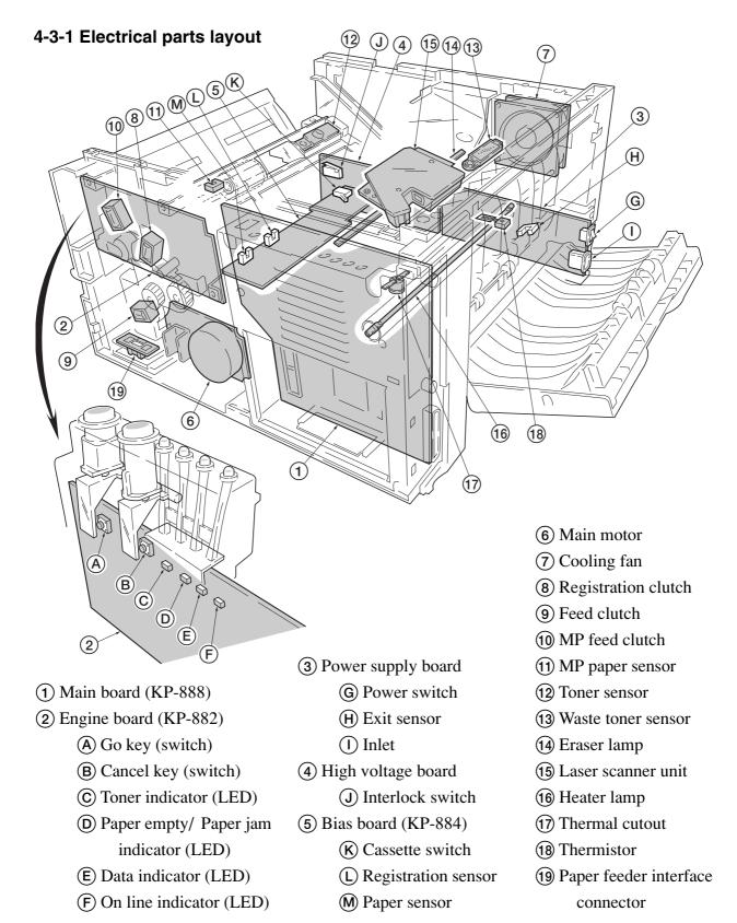
Figure 4-3-1 Electrical parts layout
