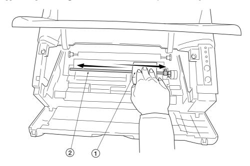
Figure 3-1-5 Cleaning the registration roller
