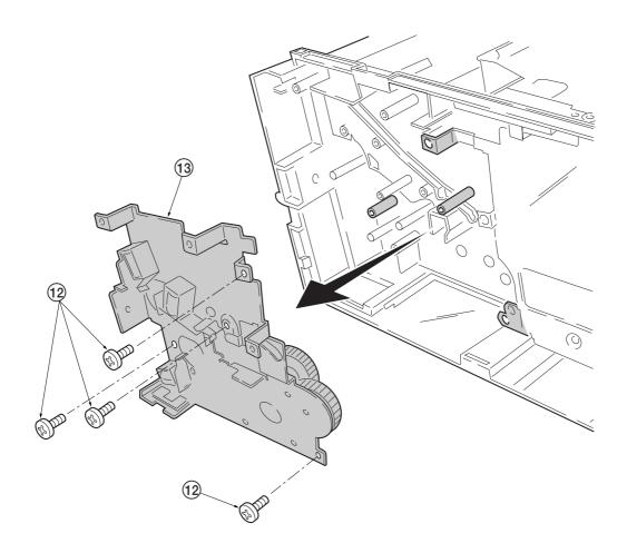
Figure 5-2-18 Removing the drive unit
