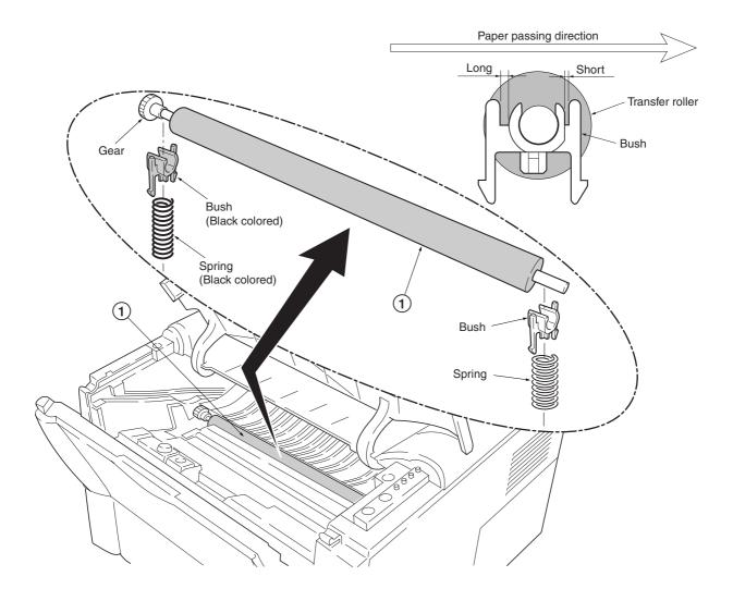
Figure 5-2-9 Removing the transfer roller
