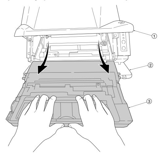
Figure 5-2-1 Removing the process unit
