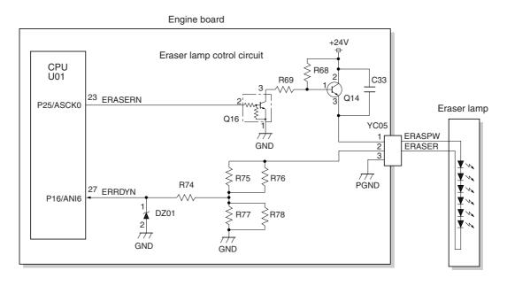
Figure 4-3-4 Eraser lamp control circuit
