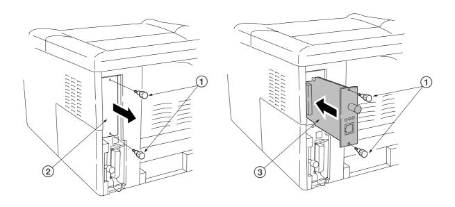
Figure 2-2-11 installing the memory card
