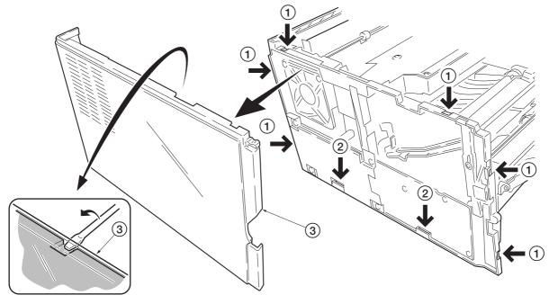
Figure 5-2-4 Removing the left cover
