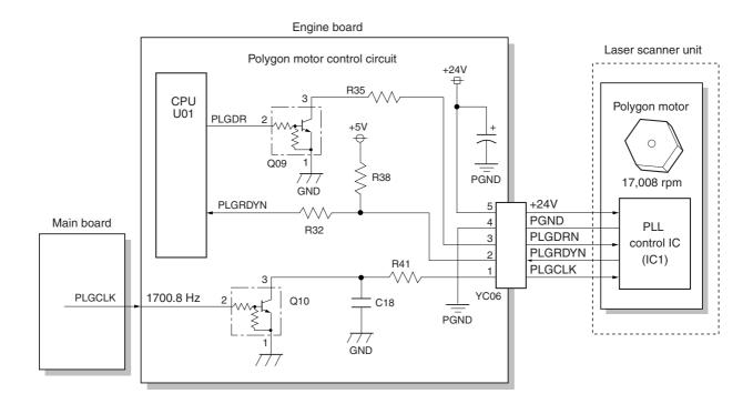
Figure 4-3-7 Polygon motor control circuit
