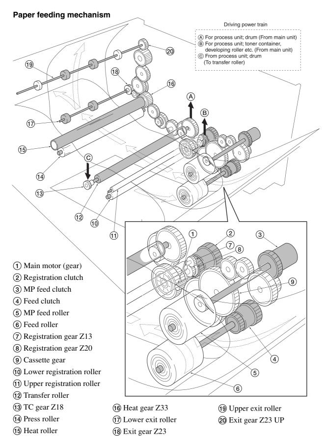
Figure 4-2-3 Paper feeding mechanism
