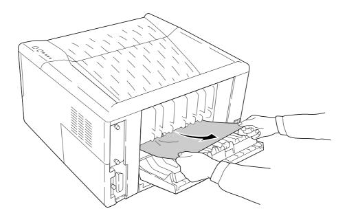
Figure 6-1-3 Jam at the face-down and face-up trays
