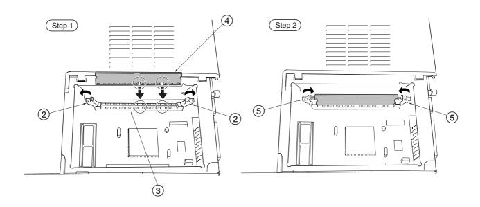
Figure 2-2-8 Inserting the DIMM
