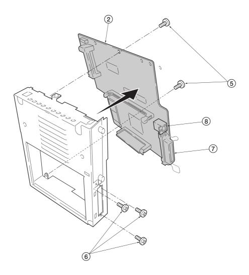
Figure 5-2-12 Removing the main board
