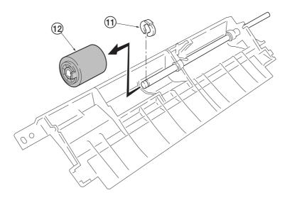
Figure 5-2-8 Removing the MP feed roller
