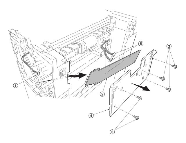
Figure 5-2-14 Removing the bias board
