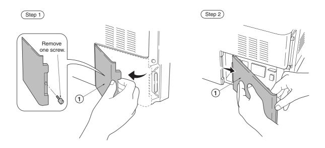
Figure 2-2-7 Removing side cover
