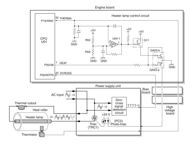
Figure 4-3-5 heater lamp control circuit
