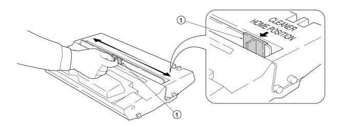
Figure 3-1-6 Cleaning the main charger wire
