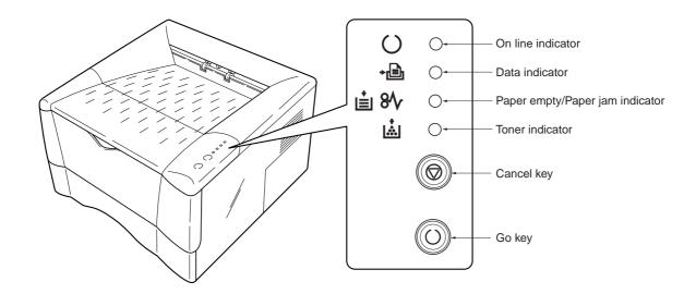
Figure 6-1-1 Indicators and control keys
