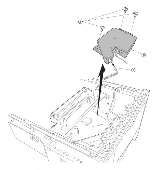
Figure 5-2-27 Removing the laser scanner unit
