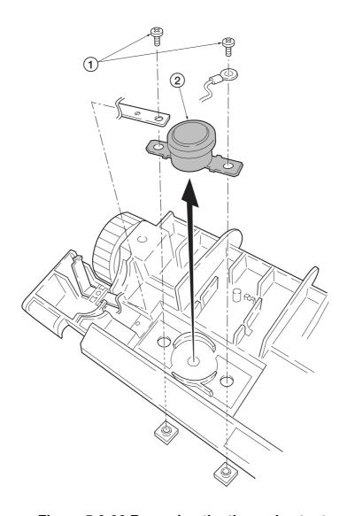
Figure 5-2-26 Removing the thermal cutout
