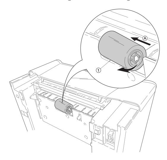
Figure 5-2-5 Removing the feed roller
