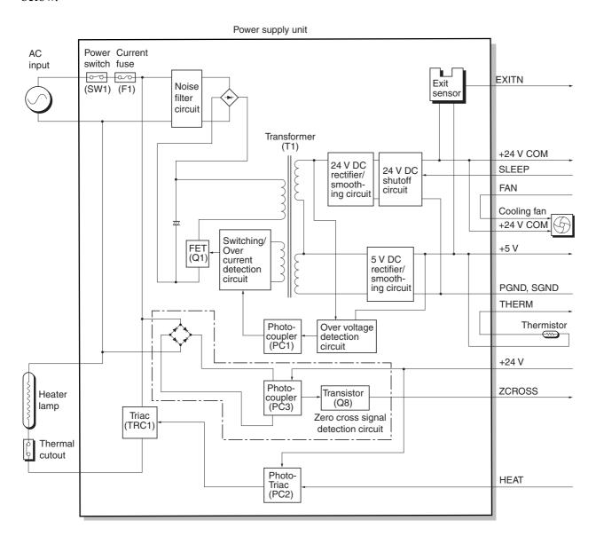
Figure 4-3-8 Power supply board circuit block diagram
