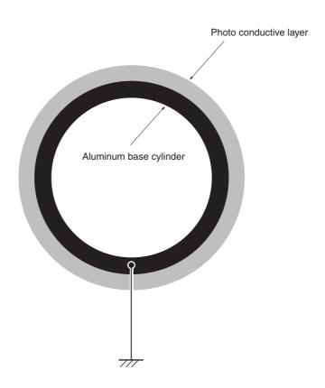
Figure 4-1-3 Photo conductive drum
