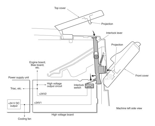
Figure 4-3-11 Interlock switch
