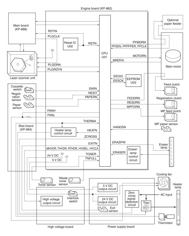
Figure 4-3-3 Engine board circuit block diagram
