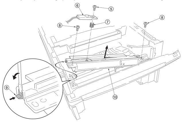
Figure 5-2-7 Removing the MP feed unit
