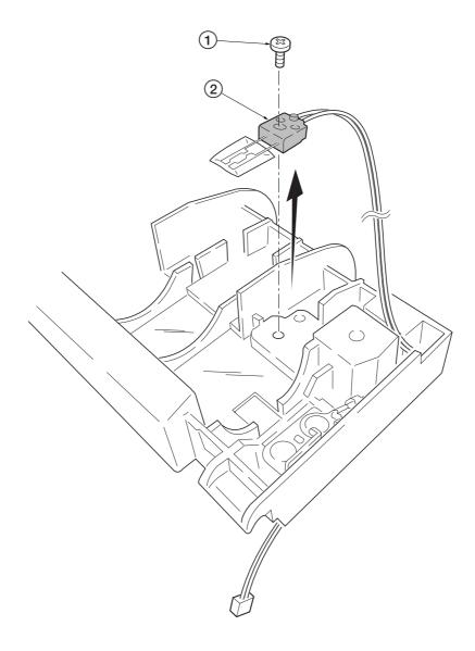
Figure 5-2-25 Removing the thermistor
