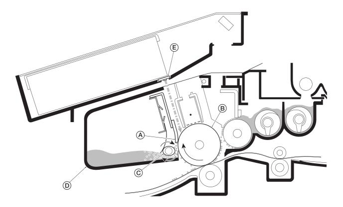
Figure 4-1-12 Drum cleaning and erasing static charge
