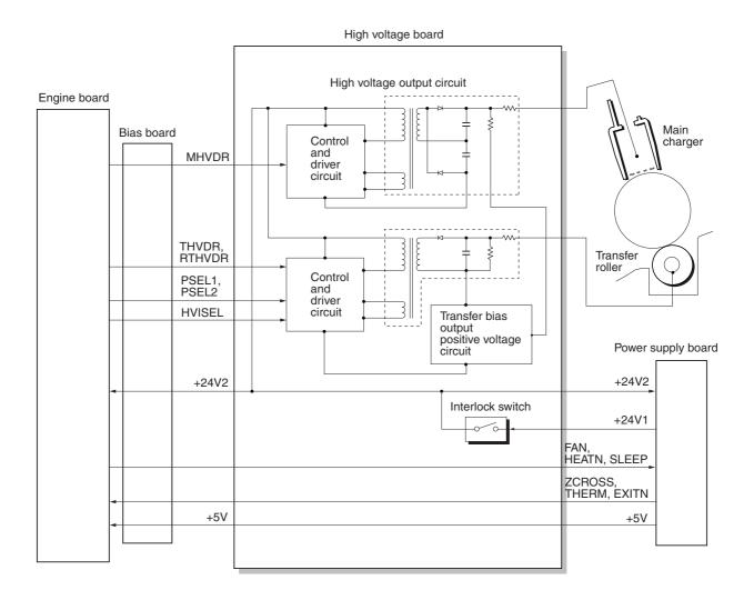
Figure 4-3-10 High voltage board circuit block diagram
