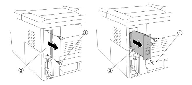
Figure 2-2-9 Removing the option interface slot cover
