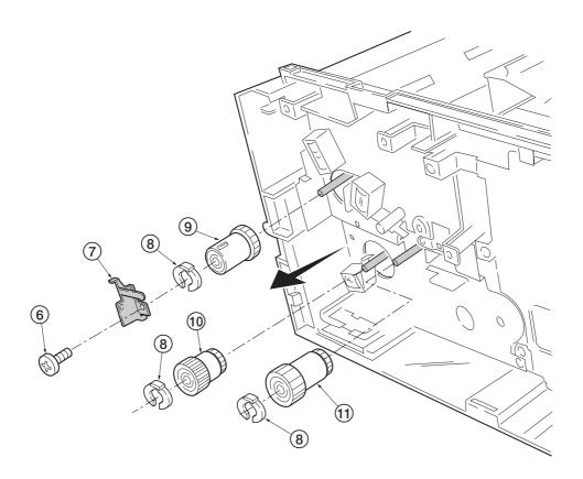
Figure 5-2-17 Removing the clutches
