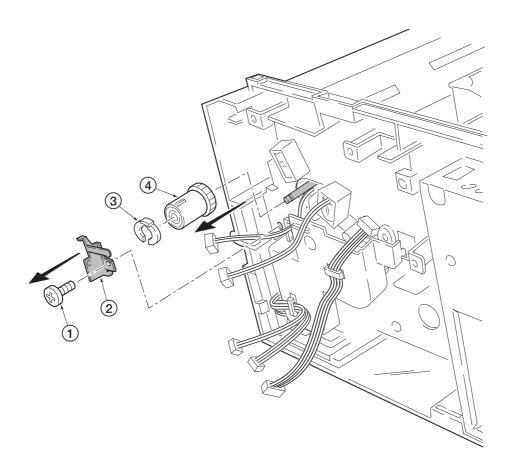
Figure 5-2-6 Removing the MP feed clutch
