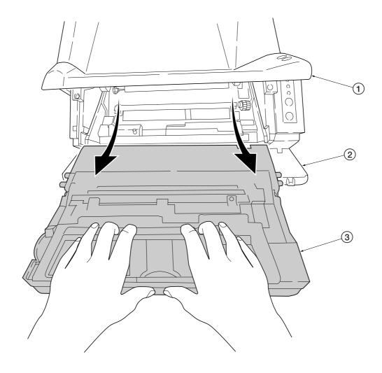
Figure 3-1-4 Removing the process unit
