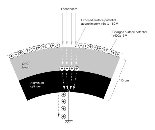
Figure 4-1-7 Drum surface potential
