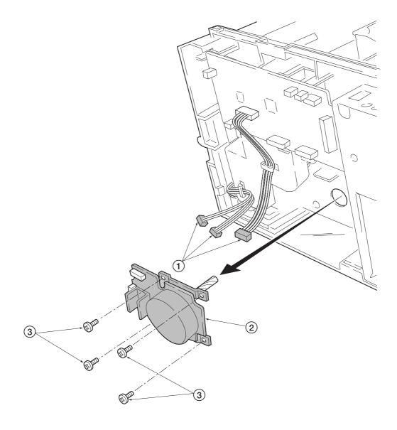
Figure 5-2-15 Removing the main motor
