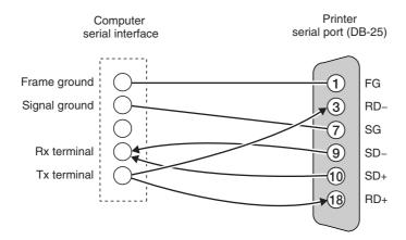
On the computer serial port, investigate pin assignments depends on the computer manufacture's instruction. Since the RS-422A configuration does not employ control lines except for data transmission/reception, select a mode in which signals such as DTR are not used.
