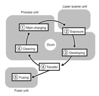
Figure 4-1-1 Electrophotographic cycle
