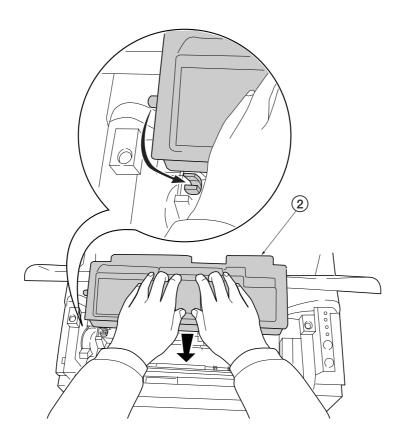
Figure 2-2-4 Installing the toner container
