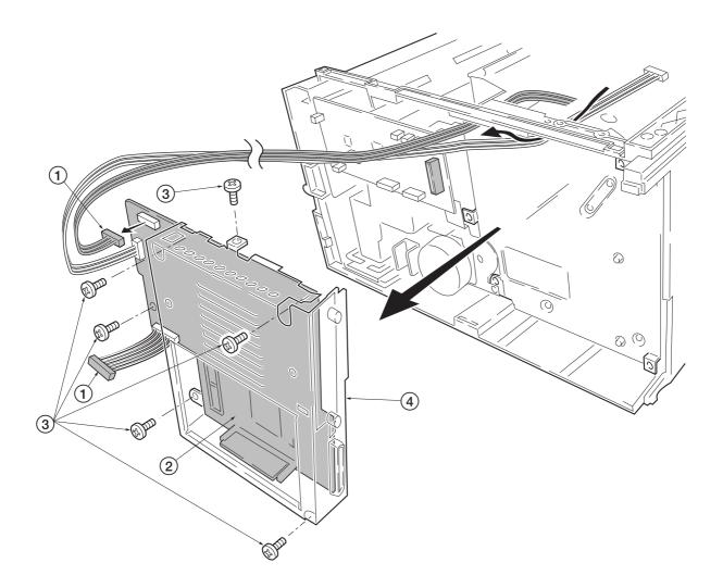
Figure 5-2-11 Removing the controller box (with main board)
