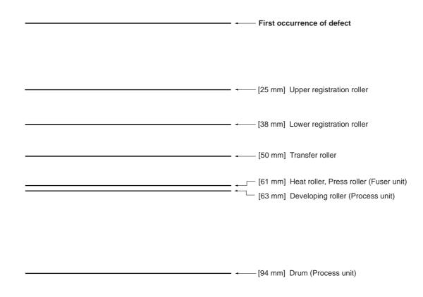
Figure 6-1-2 Repetitive defects gauge
