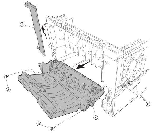
Figure 5-2-19 Removing the fuser unit
