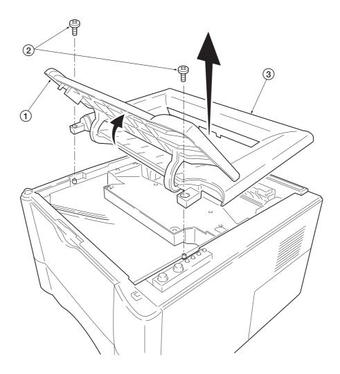
Figure 5-2-2 Removing the top cover/face-down output tray
