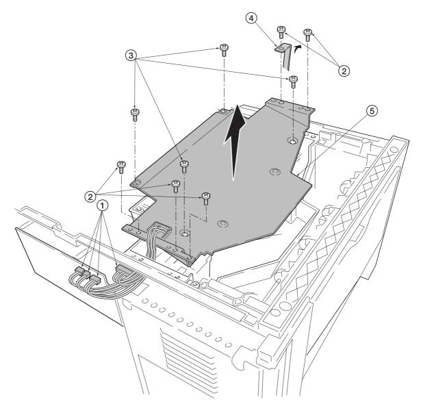
Figure 5-2-28 Removing the LSU plate
