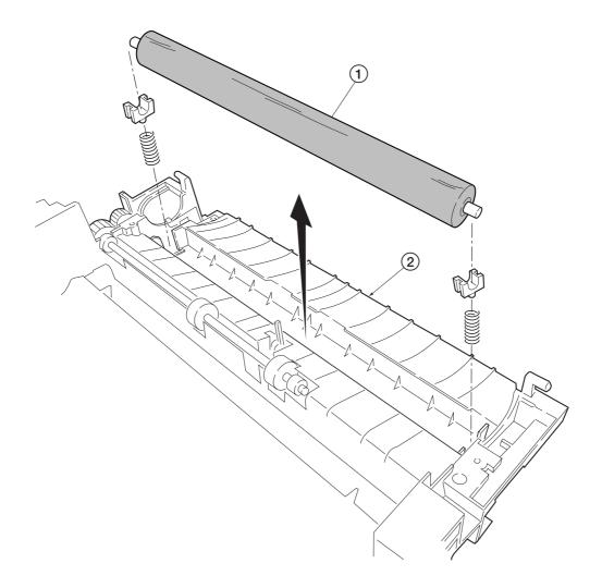
Figure 5-2-27 Removing the press roller
