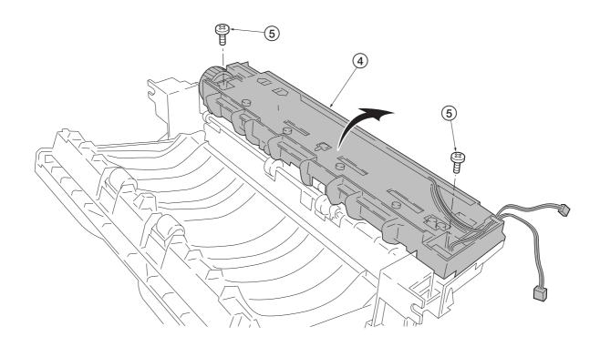
Figure 5-2-20 Splitting the fuser unit
