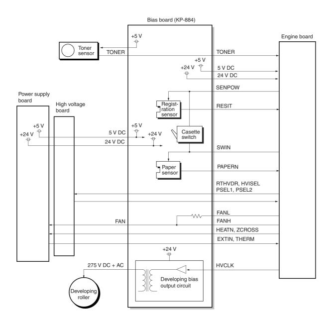
Figure 4-3-9 Bias board circuit block diagram
