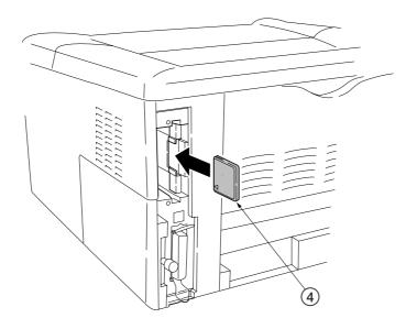
Figure 2-2-10 installing the memory card
