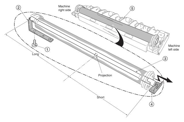
Figure 5-2-22 Removing the heater lamp
