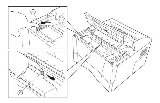
Figure 3-1-1 Releasing Lock levers #1 and #2
