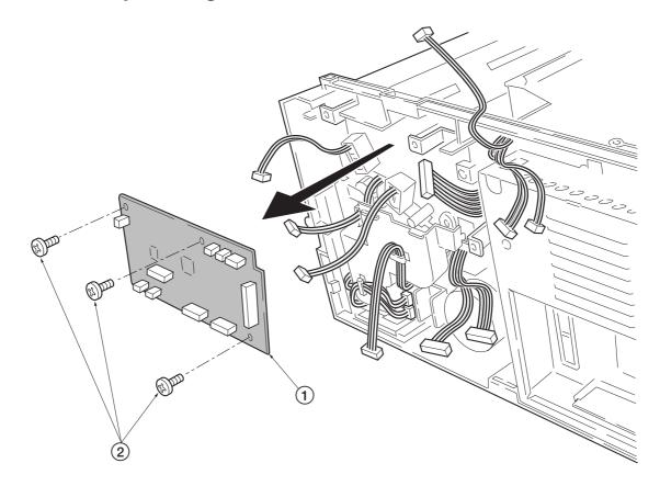
Figure 5-2-10 Removing the engine board
