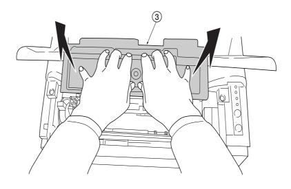
Figure 3-1-2 Removing the old toner container
