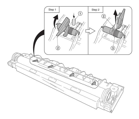
Figure 5-2-21 Removing the separators
