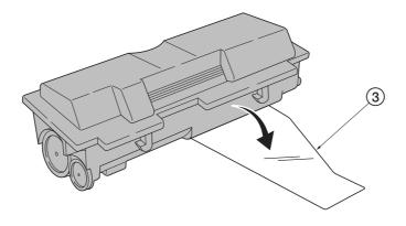
Figure 2-2-3 Removing the protective seal
