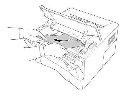
Figure 6-1-5 Jam inside the printer
