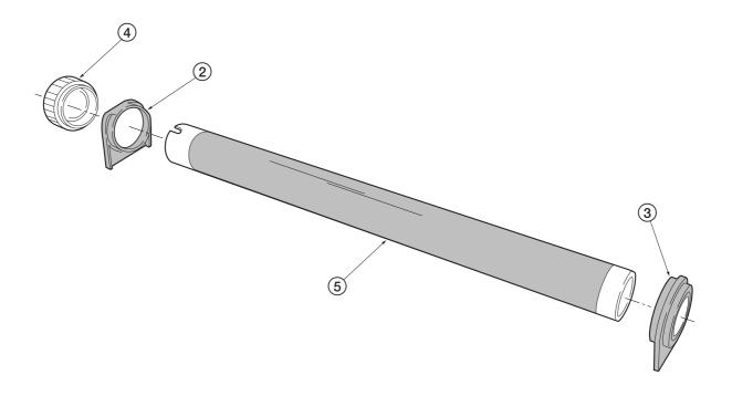
Figure 5-2-24 Removing the heat roller
