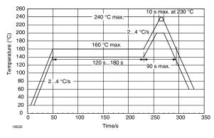
Figure 4. Recommended Solder Profile for Sn/Pb soldering
