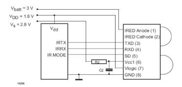
Figure 2. Typical application circuit
