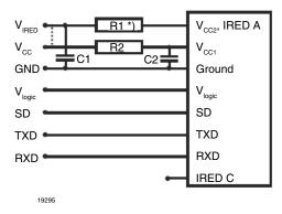
Figure 1. Recommended Application Circuit
