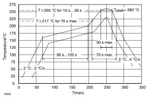
Figure 5. Solder Profile, RSS Recommendation
