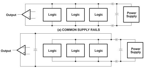
(b) SEPARATE BYPASSED SUPPLY RAILS (preferred)
