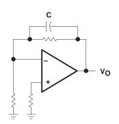
Figure 43. Compensation for Input Capacitance
