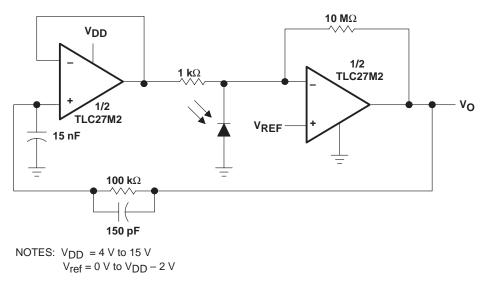
Figure 47. Photo-Diode Amplifier With Ambient Light Rejection
