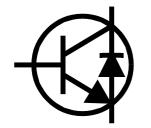
For NPN transistors, the anode of the diode is connected to the emitter of the transistor. For PNP transistors, the anode of the diode is connected to the collector of the transistor. Additionally, many Darlingtons and a few non-Darlington transistors also have a resistor shunt network between the base and emitter of the device.
