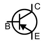
Bipolar Junction **Transistors** are available in two main types, NPN and PNP. In this example, the unit has detected a Silicon PNP transistor.
