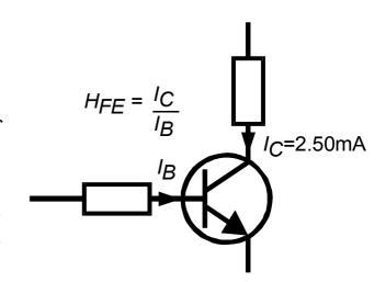
The gain of all transistors can vary considerably with collector current, collector voltage and also temperature. The displayed value for gain therefore
