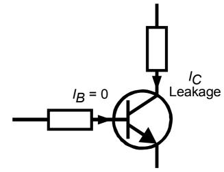
Leakage current Ic=0.17mA
