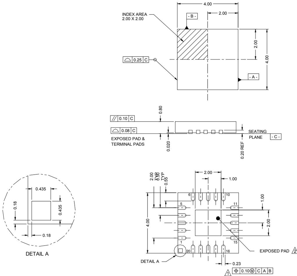
1. Dimension applies to metallized terminal and is measured between 0.25 and 0.30 from terminal tip.
