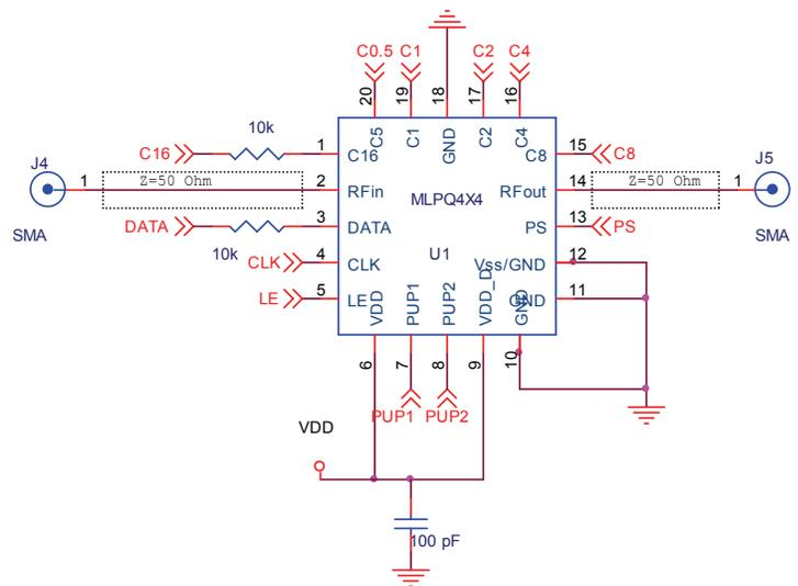
Note: Resistors on pins 1 and 3 are required to avoid package resonance and meet error specifications over frequency.
