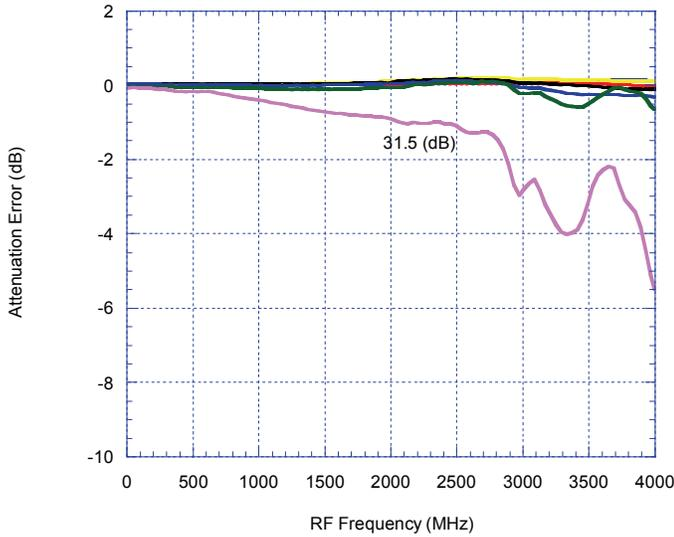
Figure 8. Attenuation Error Vs. Attenuation Setting
