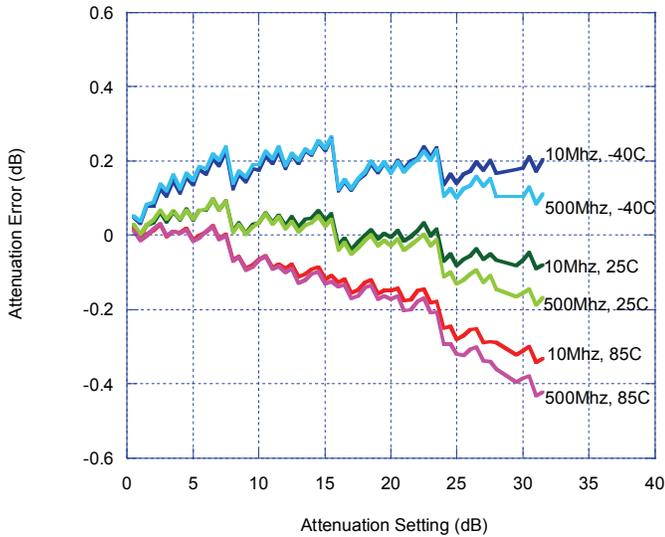
Figure 10. Attenuation Error Vs. Attenuation Setting
