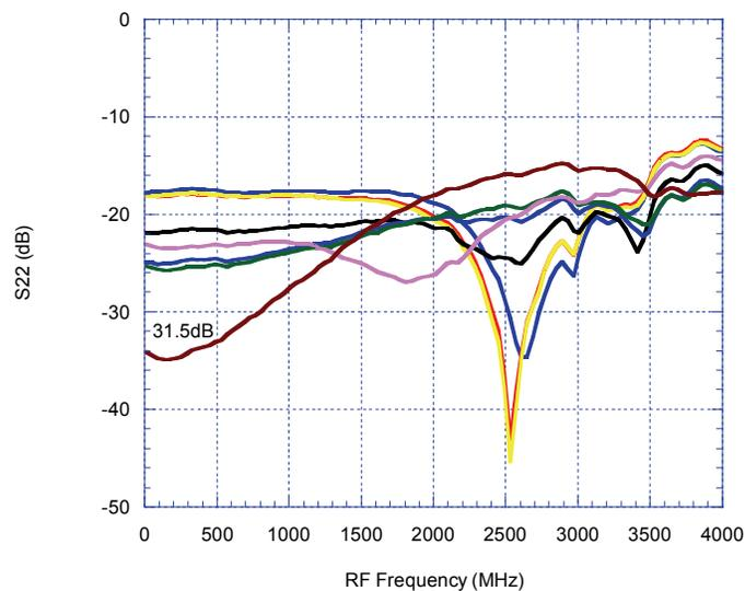
Typical Performance Data @ 25°C, V<sub>DD</sub> = 3.0 V
