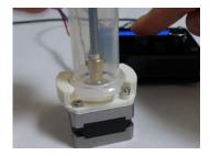
Unlock the syringe by twisting it counterclockwise. Line it up and press the left knob to lift it up.
