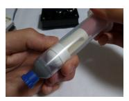
Push the piston inside while squeezing the sides of the barrel with the other hand. Trapped air will escape through the small gap between the syringe walls and the piston, you can feel when this is happening.
