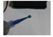
The tips themselves can also be cleaned: remove the paste with a toothpick and then with a rolled up napkin wipe the inside, a couple of drops of isopropyl alcohol help a lot.
