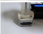
Then thread the barrel in the shaft of the motor as far down as you can.
