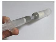
Remember to place the piston all the way in before transferring the paste, this will prevent air from getting trapped inside.
