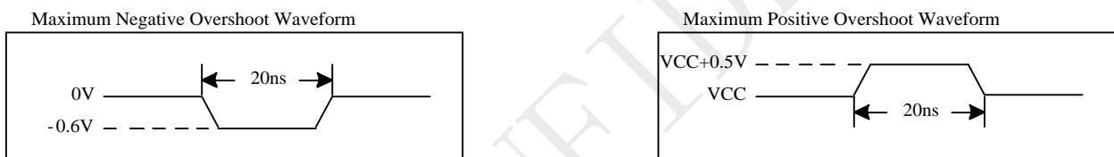
Figure 5-1 Maximum Overshoot Waveform
