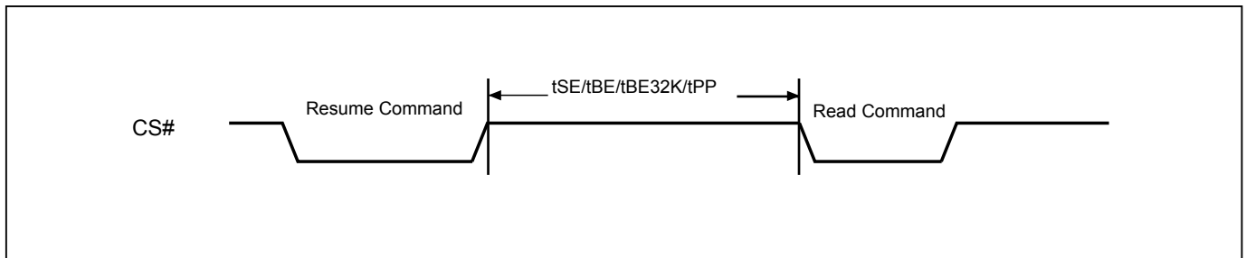
Figure 57. Resume to Read Latency
