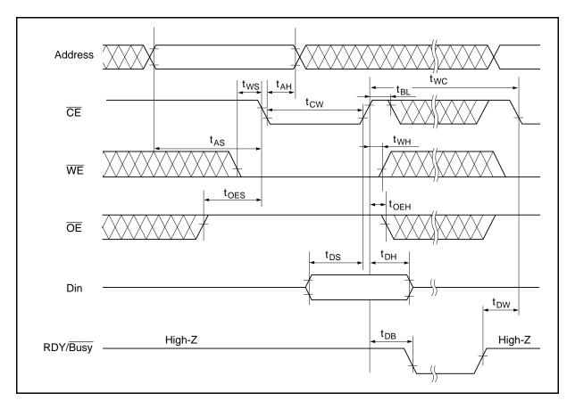
Byte Write Timing Waveform (2) (TE Controlled)
