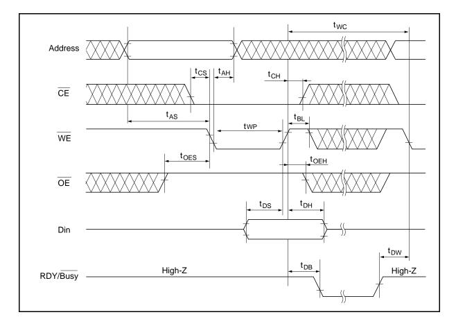
Byte Write Timing Waveform (1) (WE Controlled)
