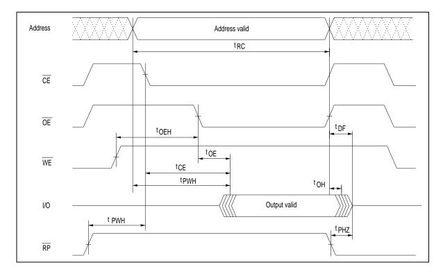
Read Timing Waveform (Byte Mode or Word Mode)
