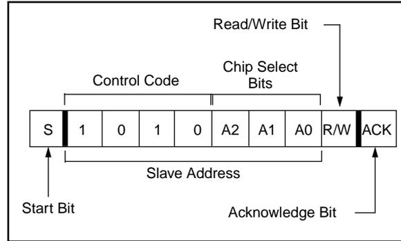
**FIGURE 5-2: ADDRESS SEQUENCE BIT ASSIGNMENTS**
