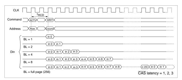
**2. Single write:** A single write operation is enabled by setting OPCODE (A9, A8) to (1, 0). In a single write operation, data is only written to the column address (AY0 to AY7) and the bank select address (A9) specified by the write command set cycle without regard to the burst length setting. (The latency of data input is 0).
