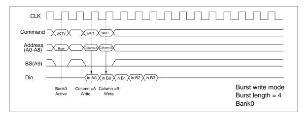
**2.** Same bank, different ROW address: When the ROW address changes, consecutive write commands cannot be executed; it is necessary to separate the two write commands with a precharge command and a bank-active command.
