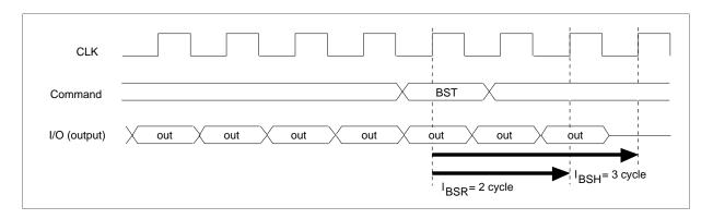
**Burst stop command at burst write:** The burst stop command (BST command) is used to stop data input during a full-page burst write. No data is written in the same cycle as the BST command and in subsequent cycles.
