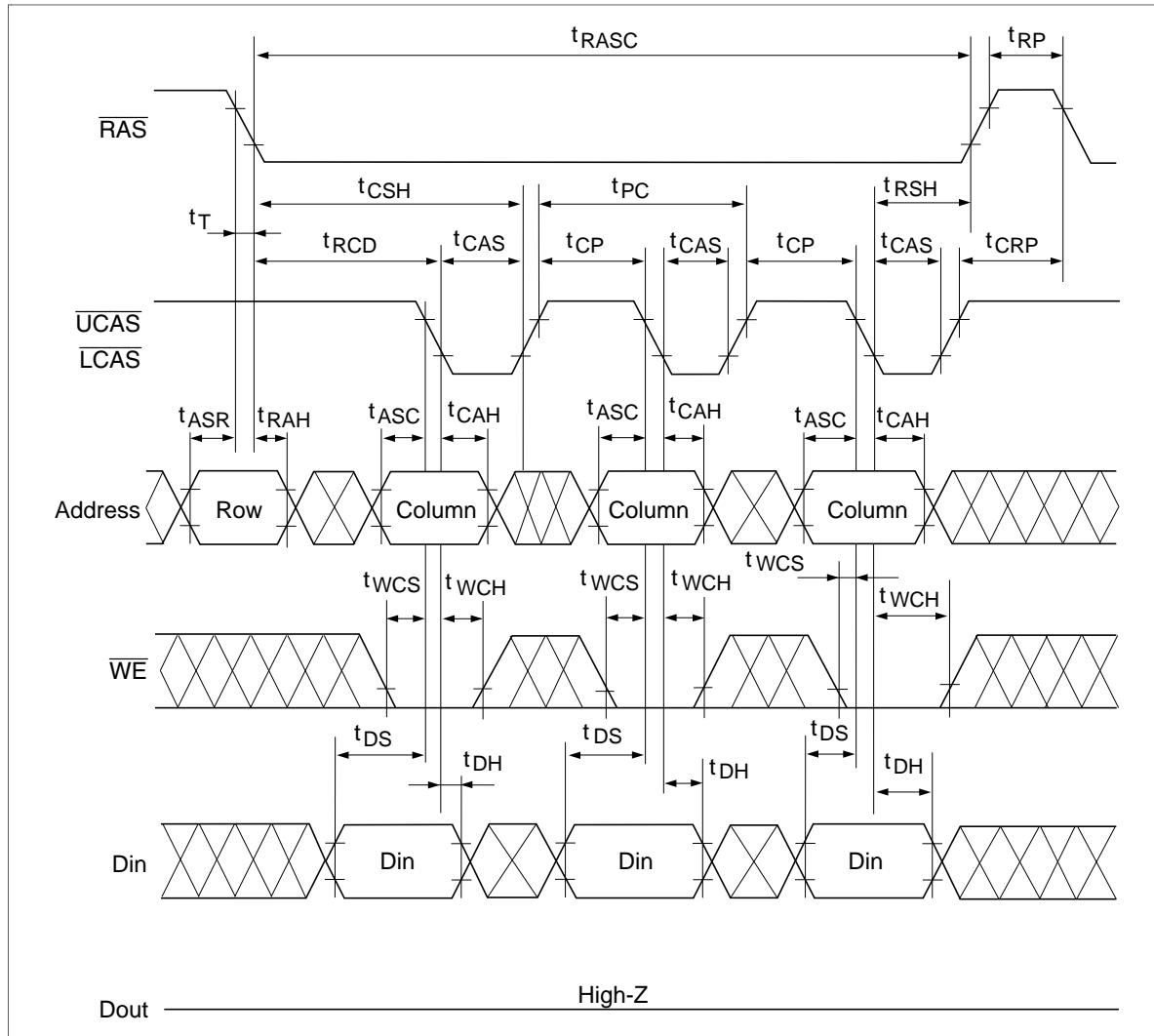
**Fast Page Mode Delayed Write Cycle**
