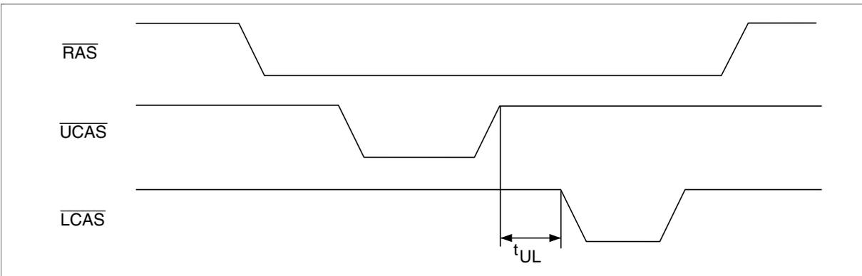
4. Byte control operation by remaining  $\overline{UCAS}$  or  $\overline{LCAS}$  high is guaranteed.
