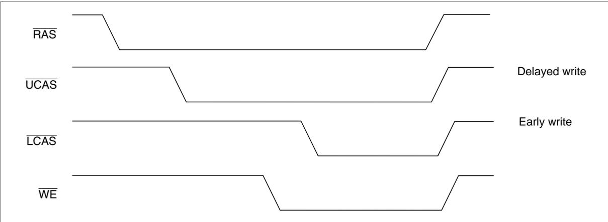
3. Closely separated upper/lower byte control is not allowed. However when the condition ( $t_{CP} \leq t_{UL}$ ) is satisfied, EDO page mode can be performed.
