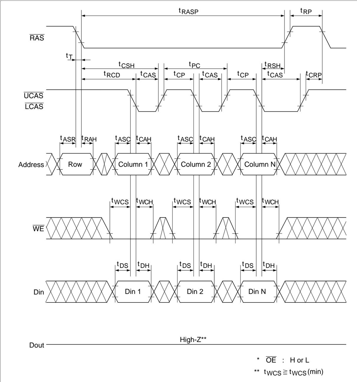
Fast Page Mode Delayed Write Cycle<sup>\*19</sup>
