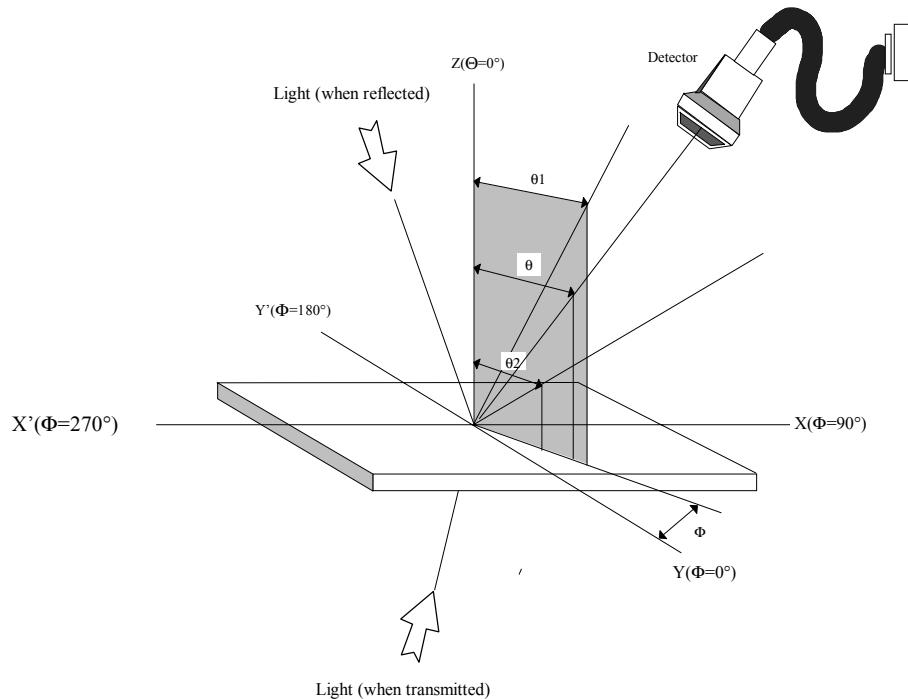
$$\text{Definition of contrast Cr.} \quad Cr. = \frac{B_1}{B_2} = \frac{\text{Brightness of not selected segm ent}}{\text{Brightness of selected segm ent}}$$
