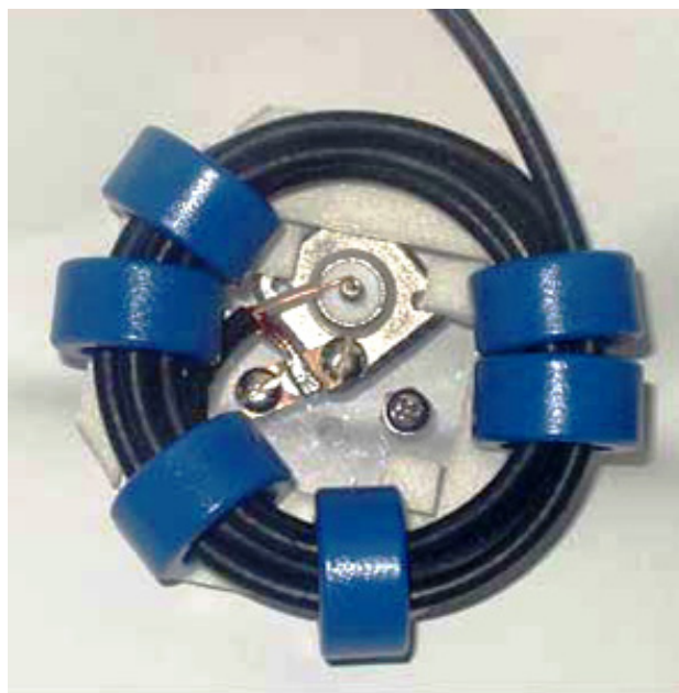
Figure 8 Simple common-mode suppression choke construction
