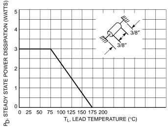
Figure 5. Steady State Power Derating
