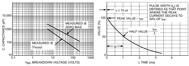
Figure 3. Capacitance versus Breakdown Voltage
