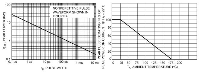
Figure 1. Pulse Rating Curve
