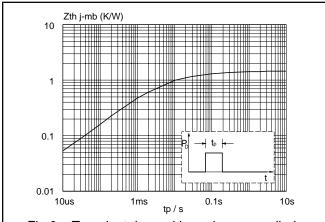
Fig.6. Transient thermal impedance per diode;  $Z_{th j\text{-}mb} = f(t_p)$ .
