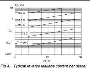
*Ig.4.* Typical reverse leakage current per diode  $I_R = f(V_R)$ ; parameter  $T_j$
