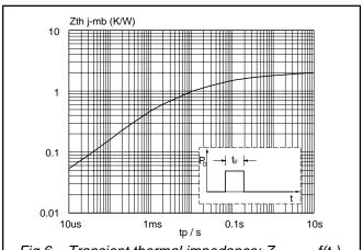
Fig.6. Transient thermal impedance;  $Z_{th j-mb} = f(t_p)$ .
