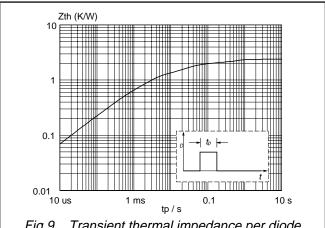
Fig.9. Transient thermal impedance per diode  $Z_{th j-mb} = f(t_p)$
