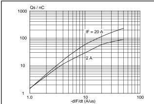
Fig.8. Maximum  $Q_s$  at  $T_i = 25^{\circ}C$ ; per diode
