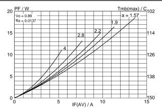
Fig.4. Maximum forward dissipation  $P_F = f(I_{F(AV)})$  per diode; sinusoidal current waveform where a = f form factor  $= I_{F(RMS)} / I_{F(AV)}$ .
