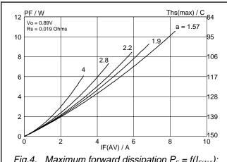
Fig.4. Maximum forward dissipation  $P_F = f(I_{F(AV)})$ ; sinusoidal current waveform where a = form factor =  $I_{F(RMS)} / I_{F(AV)}$ .
