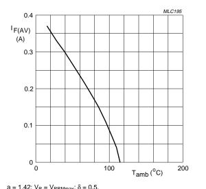
$a=1.42;\ V_R=V_{RRMmax};\ \delta=0.5.$  Device mounted as shown in Fig.11. Switched mode application.
