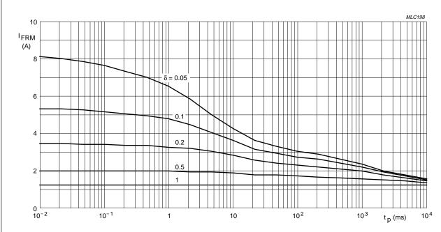
$T_{tp}$  = 85 °C;  $R_{th j-tp}$  = 30 K/W.
