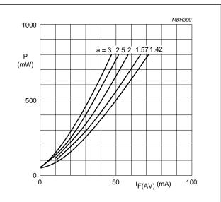
$a = I_{F(RMS)}/I_{F(AV)}; \ \delta = 0.5; \ V_R = V_{RWmax}.$
