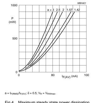
Fig.4 Maximum steady state power dissipation (forward plus leakage losses) as a function of average forward current.
