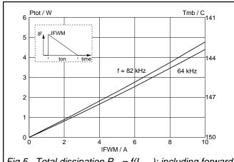
Fig.5. Total dissipation  $P_{tot} = f(I_{FWM})$ ; including forward recovery losses; Basic horizontal deflection circuit.
