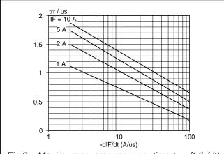
Fig.8. Maximum reverse recovery time  $t_{rr} = f(dI_F/dt)$ ; parameter  $T_j$ ;  $V_R \ge 30V$
