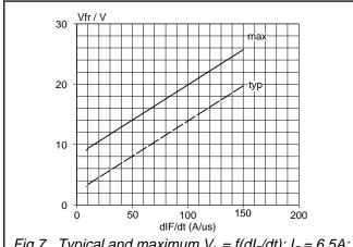
Fig.7. Typical and maximum  $V_{fr} = f(dI_F/dt)$ ;  $I_F = 6.5A$ ;  $T_j = 25 \degree C$
