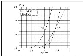
Fig.6. Typical and maximum forward characteristic  $I_F = f(V_F)$ ; parameter  $T_i$
