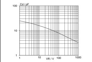
Fig.8. Typical junction capacitance  $C_d$  at f = 1 MHz,  $T_j = 25^{\circ}C$
