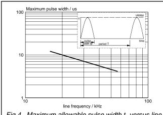
Fig.4. Maximum allowable pulse width t<sub>p</sub> versus line frequency; Basic horizontal deflection circuit.
