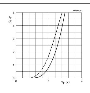
Dotted line:  $T_j = 150 \,^{\circ}\text{C}$ . Solid line: T<sub>i</sub> = 25 °C.
