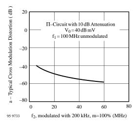
Figure 3: Typical Cross Modulation Distortion vs. Frequency f2
