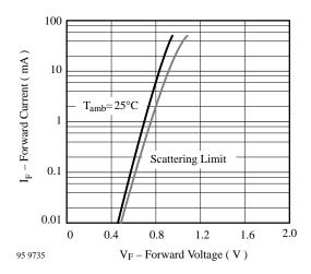
Figure 1 : Forward Current vs. Forward Voltage
