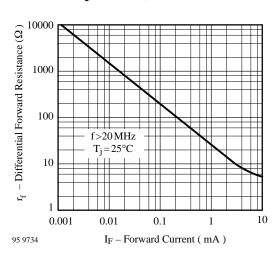
Figure 2: Differential Forward Resistance vs. Forward Current
