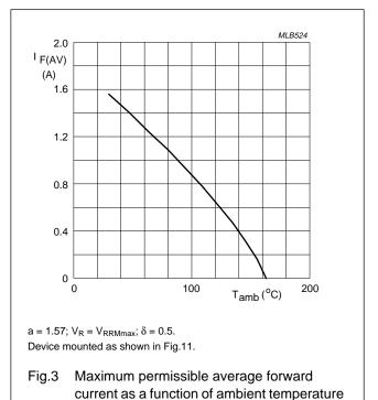
(including losses due to reverse leakage).
