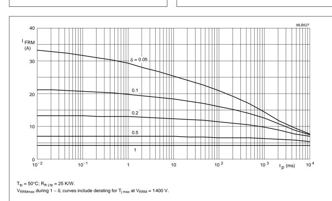
Fig.4 Maximum repetitive peak forward current as a function of pulse time (square pulse) and duty factor.
