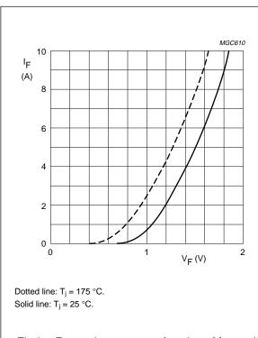
Fig.8 Forward current as a function of forward voltage; maximum values.
