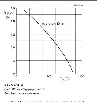
Fig.3 Maximum permissible average forward current as a function of tie-point temperature (including losses due to reverse leakage).
