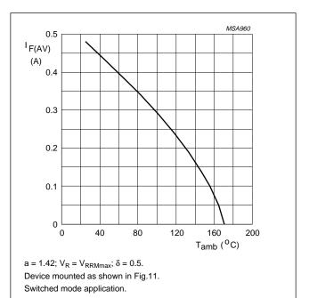
Fig.3 Maximum permissible average forward current as a function of ambient temperature (including losses due to reverse leakage).
