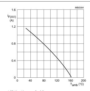
a = 1.57;  $V_R = V_{RWMmax}$ ;  $\delta$  = 0.5. Device mounted as shown in Fig.9.
