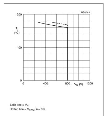
Fig.5 Maximum permissible junction temperature as a function of reverse voltage.
