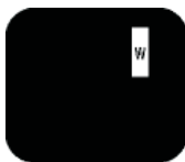
Three adjacent lit subpixels (one white pixel)
