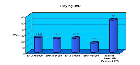
DVD playback performance of these two platforms is not only flawless but the scores are also very close to each other. In figure 2, the power consumption of the EPIA M10000 and the Fanless EPIA ME6000 is less than half of that of the reference platform.
