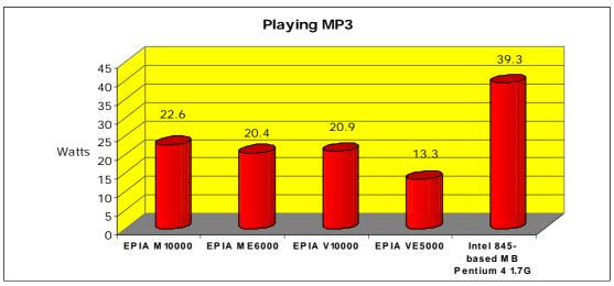
Power consumption of the fanless VIA EPIA ME6000 is around half of that of the reference platform at 51.9%. It is interesting to note that for MP3 playback the fanless VIA EPIA VE5000 only uses around 30% of the power that the reference platform uses. This is significant power sensitive systems like car MP3 players are gaining in popularity.
