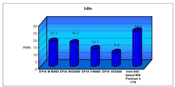
In this comparison, the power consumed while standing idle is compared and the VIA EPIA M-Series mainboards draw around 60% of the power that the reference platform draws.
