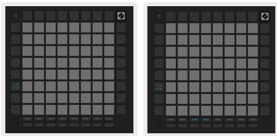
5.3.7.A – Setting the number of bars with the Track Select Buttons for Fixed Length. A fixed length of 1 bar is seen on the left image, and 4 bars on the right.
