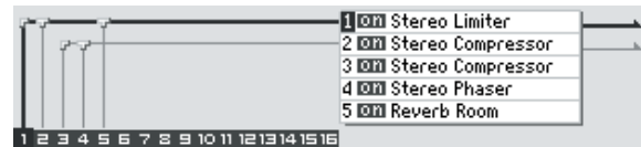
Example: Inserting a separate IFX into each timbre, and then inserting an IFX at the final stage
